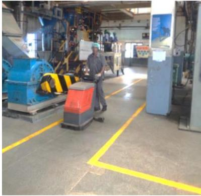
Fig.6.3.21. Special stone flooring to avoid slipping and easy to clean
