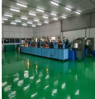
Fig.6.3.22.Epoxy and smooth flooring, easy to clean and avoids dust accumulation and microbial contamination
