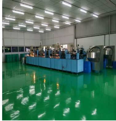
Fig.5.3.22. Epoxy and smooth flooring, easy to clean and avoids dust accumulation and microbial contamination
