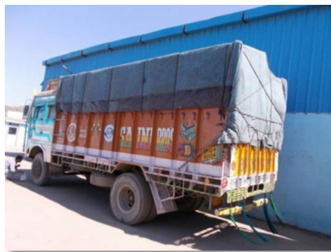
Fig.5.3.30. Multilayer Tarpaulin to protect from water and dust
