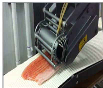
Fig. 4.3.10. Pin bone removal machine Used to extract of fish pin bones without affecting the integrity of the meat, and without breaking the pin bones, thus avoiding that parts thereof remain inserted within the fish meat
