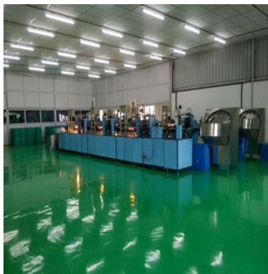
Fig.6.3.22. Epoxy and smooth flooring, easy to clean and avoids dust accumulation and microbial contamination
