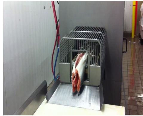
Fig. 4.3.7. Fillet processing machines Automatic fish fillet machine/fish processing machine which can fillet the fish
