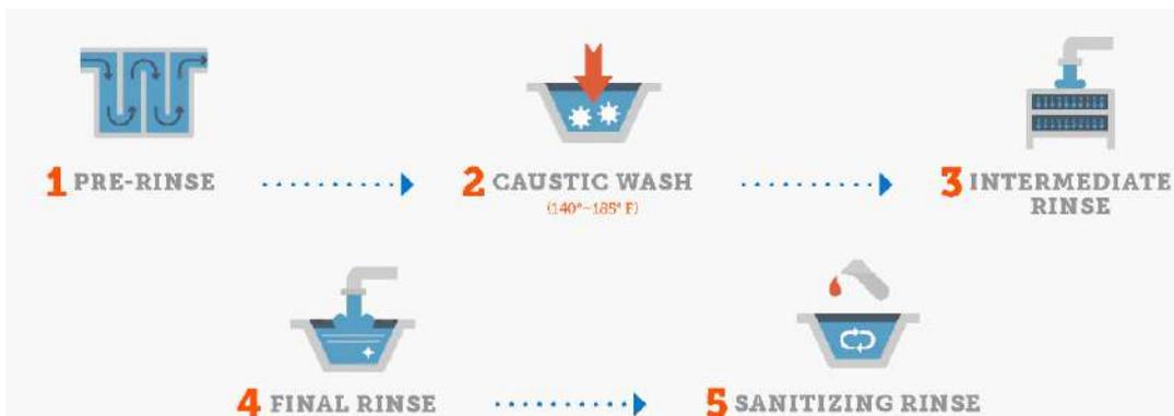
Fig. 3.3.1: Flow Diagram of CIP cycle
