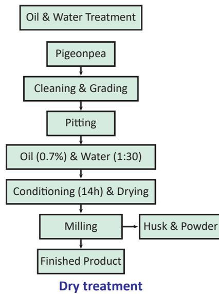
Fig. 1.3.2: Wet and Dry Treatment of Pulse Milling
