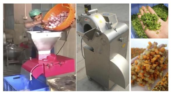
Fig. 5.1.8. Shredding/dicing/cubing/slicing machine
