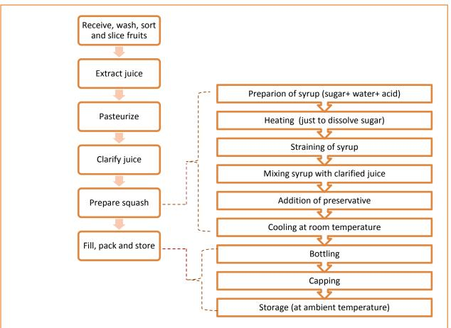
Fig.5.5.3. Squash making process for different fruit juice extra
