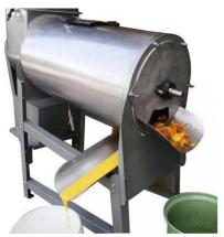
Fig. 5.2.2. Pulper Used for extraction of pulp/ juices from fruits
