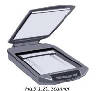
The scanner converts print data into electronic data. Images and text available in books, newspapers and magazines can be scanned and used as computer data. The scanner is similar to a photocopier machine, except here the copy comes in electronic format.
