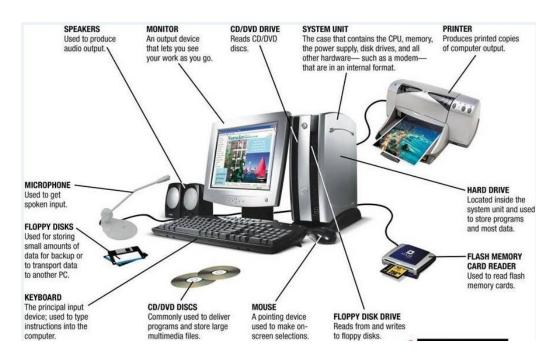
Fig. 9.1.2. Components of a Computer
