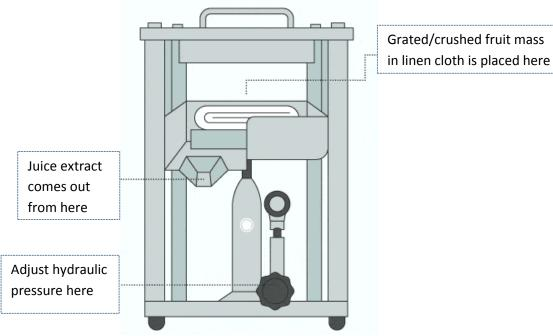
Fig. 5.2.4. Manual hydraulic press juicer Uses pressure to extract the juice out of raw produce.
