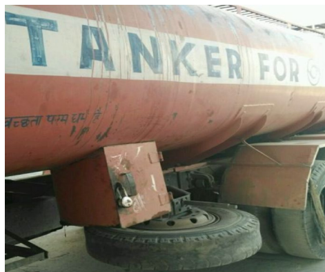
Fig.5.3.31. Display of Cleaning Status on Tankers and lock and key system provided for food defence
