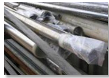
End seal for pipelines not in use
