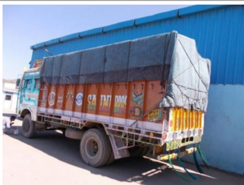
Fig.5.3.30. Multilayer Tarpaulin to protect from water and dust
