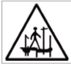
Danger Scaffolding Incomplete
