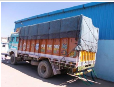
Fig.7.3.30.Multilayer Tarpaulin to protect from water and dust
