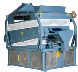
Fig. 5.3.4. De-stoner Used for removing fruit seeds and stones in fruits/vegetables
