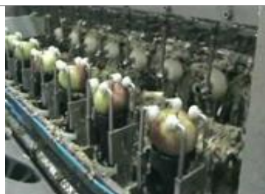
Fig. 5.3.2. Peeling machine Used for removing fruit/vegetable skin
