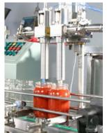
Fig .3.2.7. Pickle filling machine for bottles Used to fill processed pickles into bottles. Removes air from the bottle during the filling process
