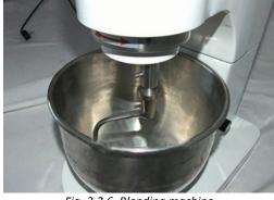
Fig. 3.2.6. Blending machine Equipped with a moving shaft that moves slowly and blends ingredients
