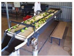
Fig. 3.2.4. Grading machine Used to grade and sort fruits/ vegetables as per size
