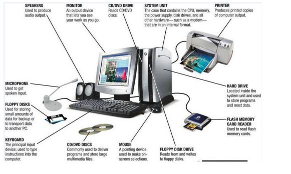
Fig.8.1.2.Components of a Computer
