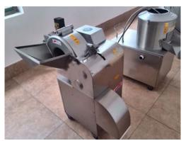
Fig. 3.2.3. Multifunction vegetable slicer/chopper Used to slice and chop vegetables, it is equipped with a chopping blade that produces fingersized cuts
