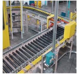
Fig.3.2.1.Roller conveyor Carries fruits and vegetables for further processes
