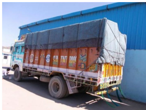
Fig.6.3.30. Multilayer Tarpaulin to protect from water and dust
