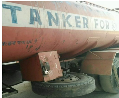
Fig.6.3.31. Display of Cleaning Status on Tankers and lock and key system provided for food defence
