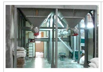
It is used to separate coarse grains and fine particles of flour using flat sieves
