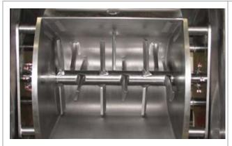
It is used to knead and mix dough for bread, bagels, pizza crusts, cake and make whipped cream, dough, icing, and fillings
