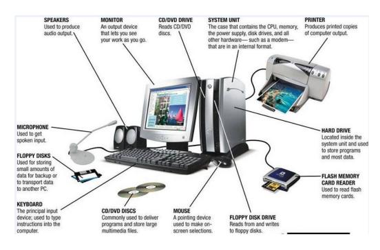
Fig. 8.1.2. Components of a Computer
