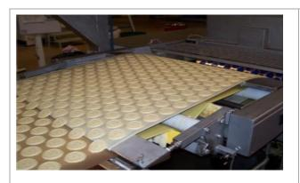
It is a pair of rollers with various shapes used for cutting the dough as per the desired shape of the biscuit
