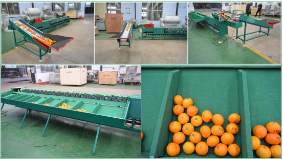
Fig.4.1.4. Sorting line conveyor
