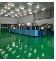
Fig.6.3.22.Epoxy and smooth flooring, easy to clean and avoids dust accumulation and microbial contamination
