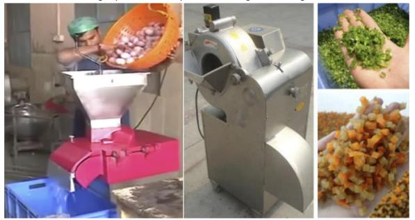
Fig. 4.2.2. Shredding/dicing/cubing/slicing machine
