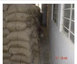
Proper stacking of raw material away from wall
