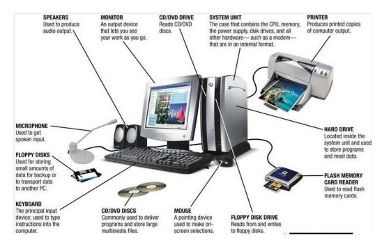
Fig. 8.1.2. Components of a Computer
