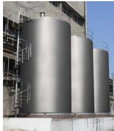
Fig. 4.1.3. Vertical insulated milk storage tank Storage tanks are containers that hold hot or cold liquids used for short or long-term storage. In the dairy industry, storage tanks are classified based on structure and heat preservation capacity
