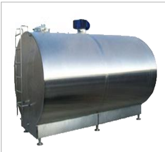
Fig. 4.1.2. Horizontal insulated milk storage tank Storage tanks are containers that hold hot or cold liquids used for short or long-term storage. In the dairy industry, storage tanks are classified based on structure and heat preservation capacity
