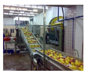
Fig. 4.2.2. Fruit/vegetable washing machine Equipped with a water holding tank that facilitates continuous water flow, used for washing fruits and vegetables
