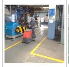
Fig.7.3.21.Special stone flooring to avoid slipping and easy to clean
