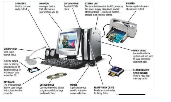
Fig. 8.1.2. Components of a Computer
