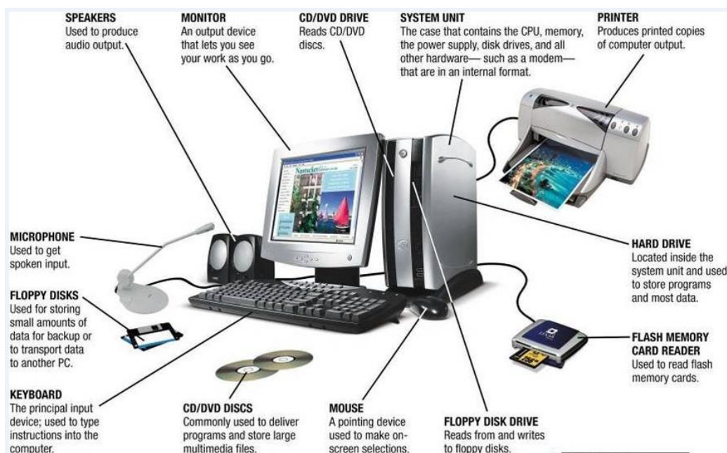
Fig. 8.1.2. Components of a Computer
