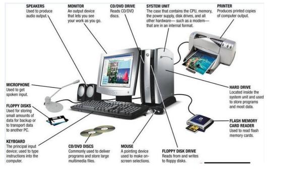
Fig. 8.1.2. Components of a Computer
