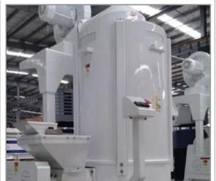
*Fig.4.1.9.Whitener* The machine provides a high quality, clean finish to the rice
