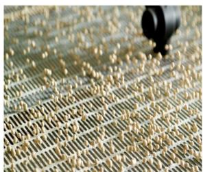
Fig.4.1.10.Thickness/width separator This machine is widely used at various largescale rice mills, seed processing plants, and grains/beans processing plants to produce high quality products because it can separate broken grains and immature grain easily and efficiently • Send the processed grains/ flour for packgaing as per the SOP (refer to the table - Types of packaging)
