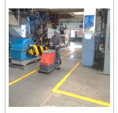
Fig.5.3.21. Special stone flooring to avoid slipping and easy to clean
