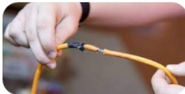
Figure 2.1.52 Damaged electrical wire
