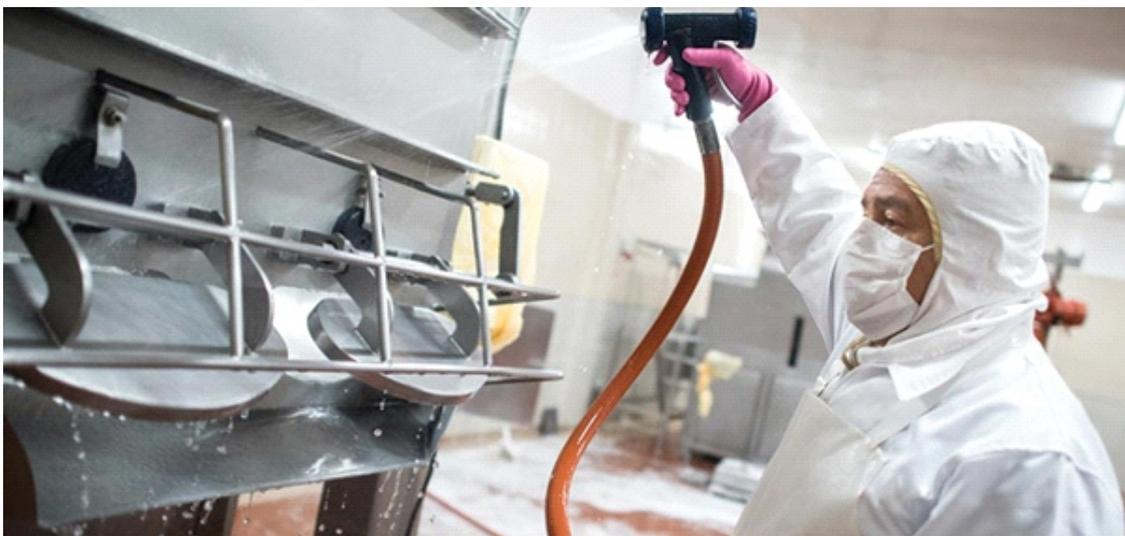
Figure 2.1.23 Pressure cleaning in Equipment (CIP)
