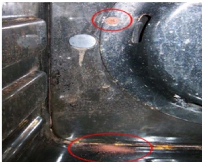
Figure 3.1.9 Patches of rust inside the oven
