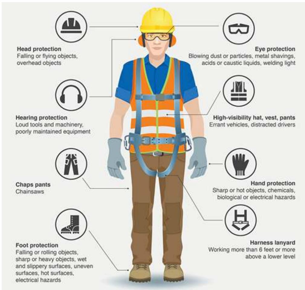
Fig. 5.5: The usage of personal protective equipment
