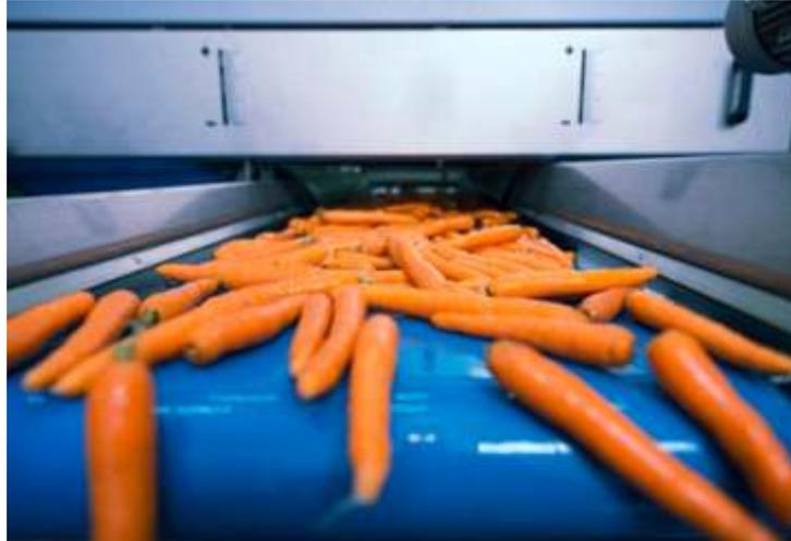
Fig.3.7 Drying line conveyor for fruits and vegetables
