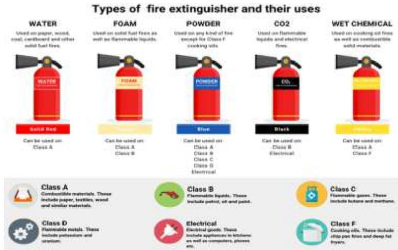
Fig. 5.7: Types of fire extinguishers
