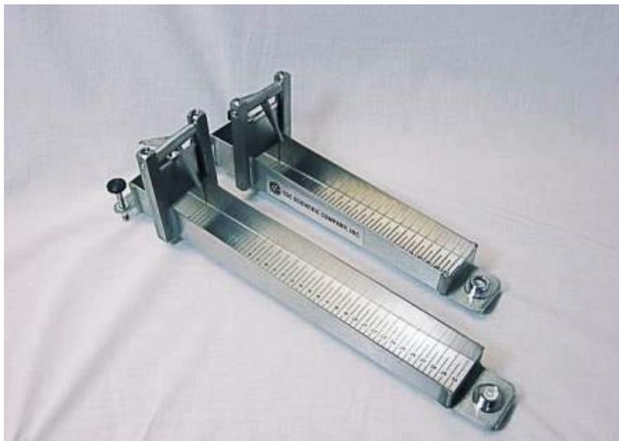
Fig 20.4 Bostwick Consistometer
