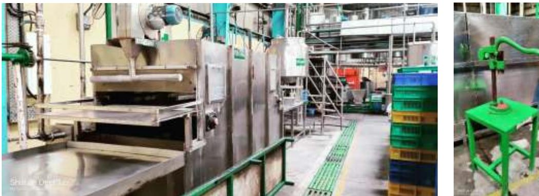
*Fig. 21.4 Cooling Machine(left) & Capping Machine(Right)*
