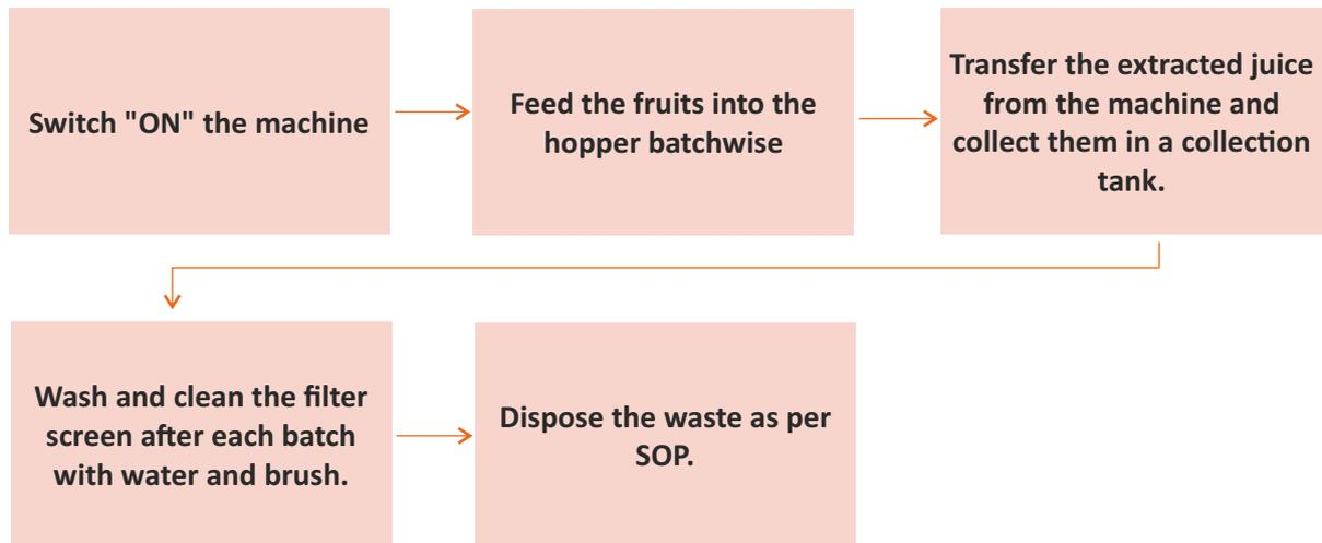
Fig. 14.4 Workflow Process of Fruit-Juice Extractor Machine
