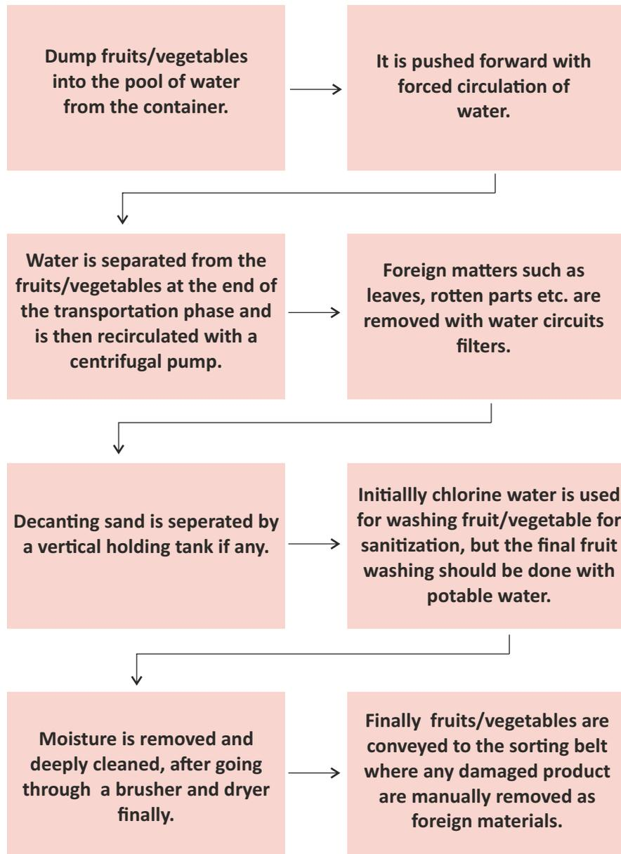
Fig.3.11 Process of drying and sorting line conveyor
