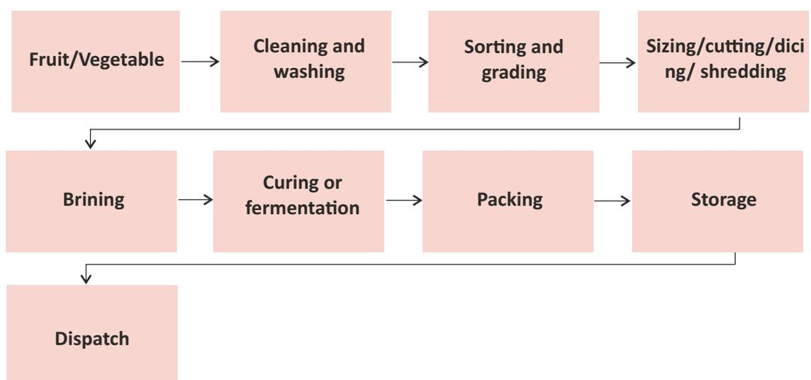
Fig.1.6 Standard Procedure for Pickle Making
