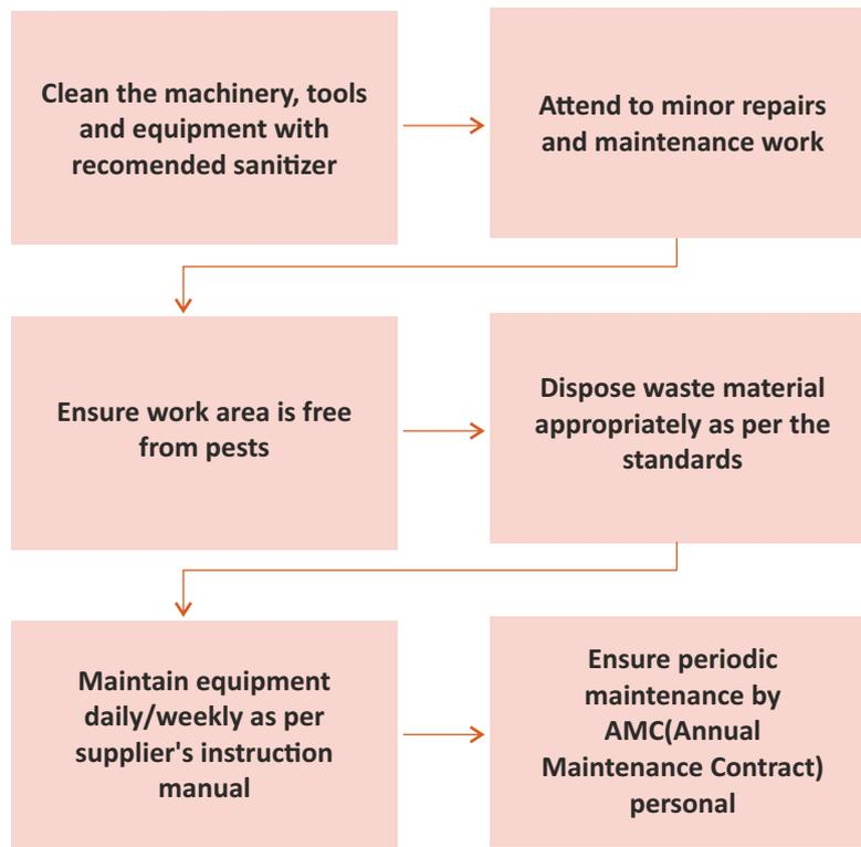
*Fig.8.7 Sequence for Cleaning Machinery and Equipment*
