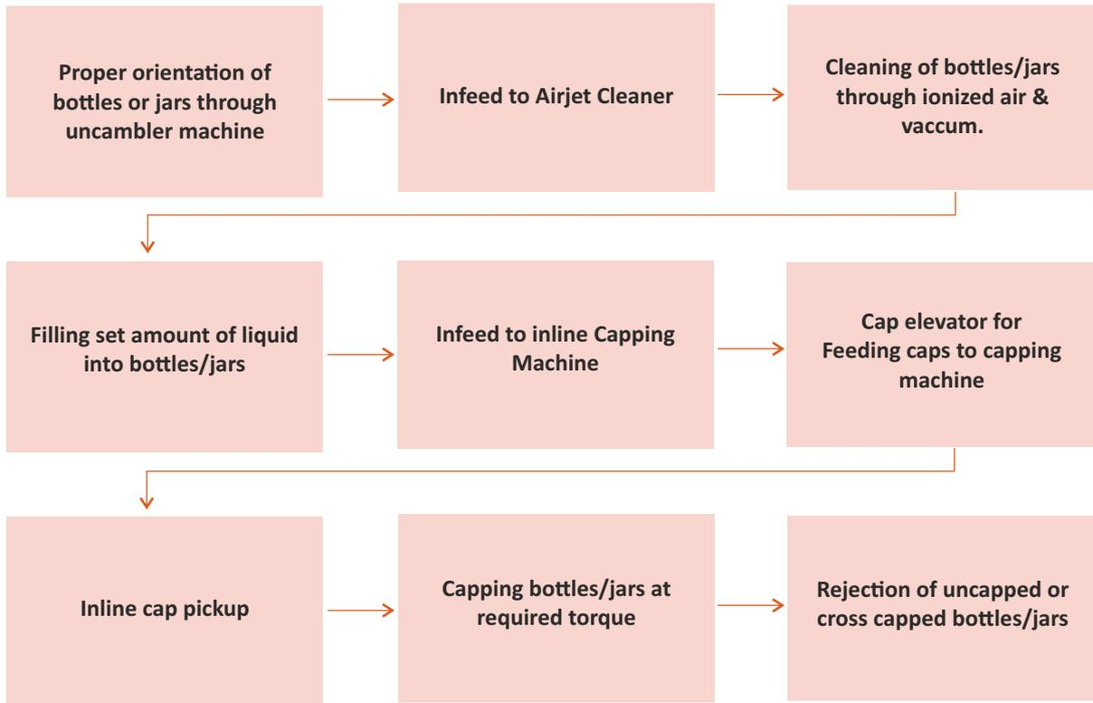
Fig. 7.5 Workflow process of Jam, Jelly and Ketchup packaging line
