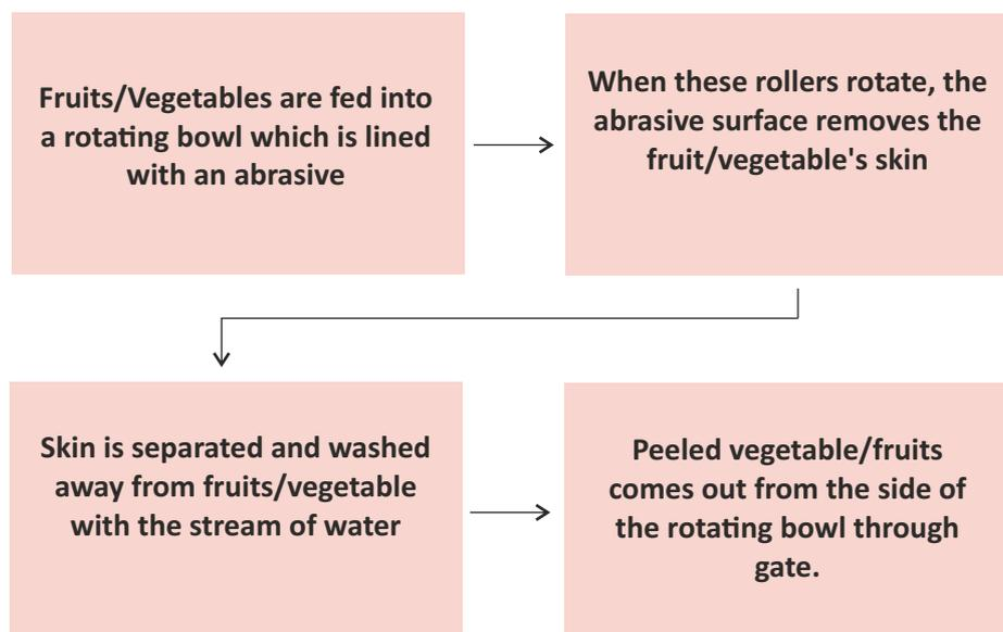
Fig. 3.14 Process of Peeling Machine
