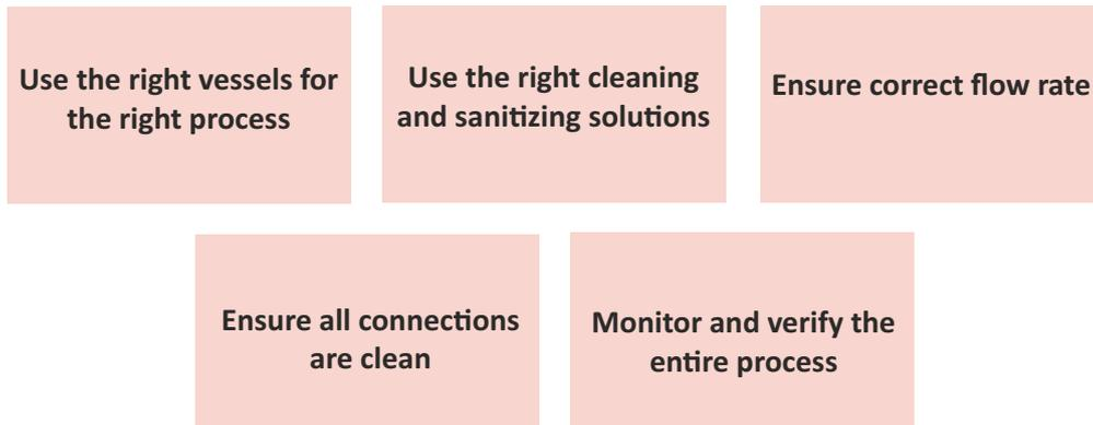
Fig 3.32 Tips for conducting an effective CIP process
