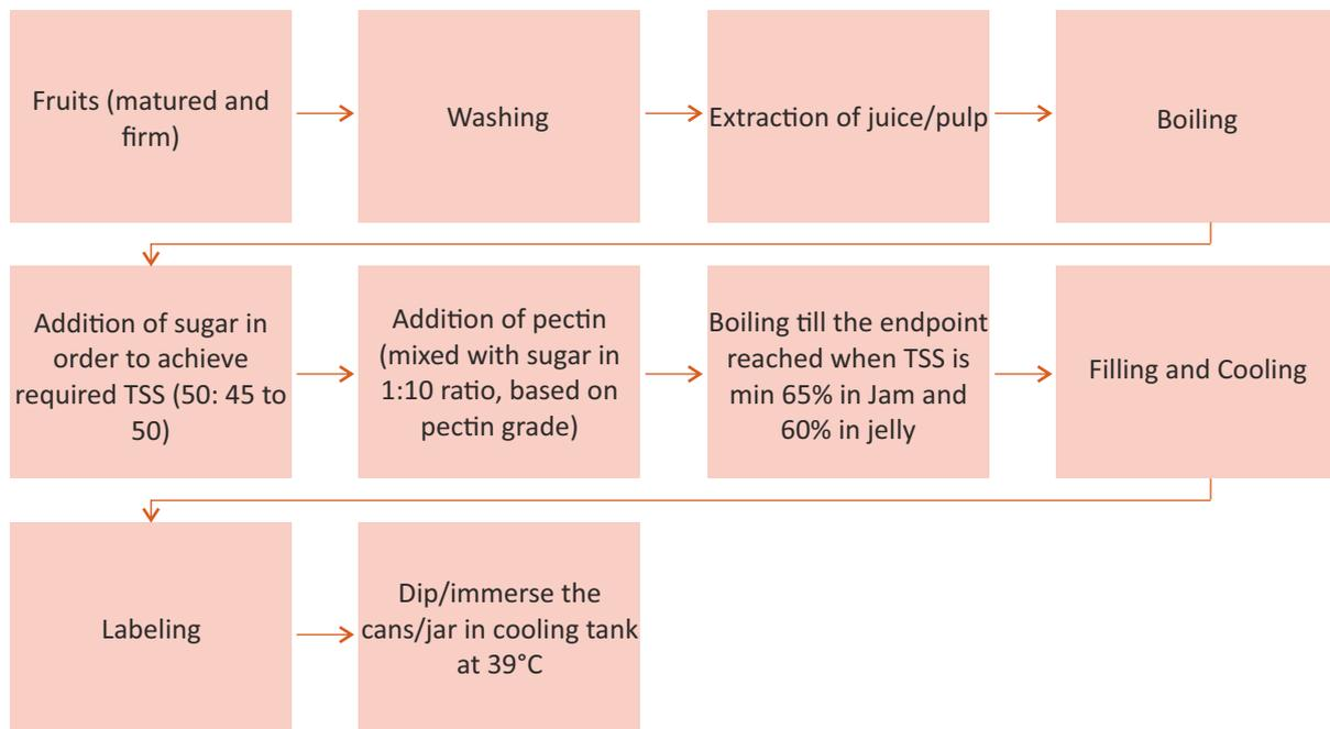
Fig.5.12 Process flowchart for preparation of jam
