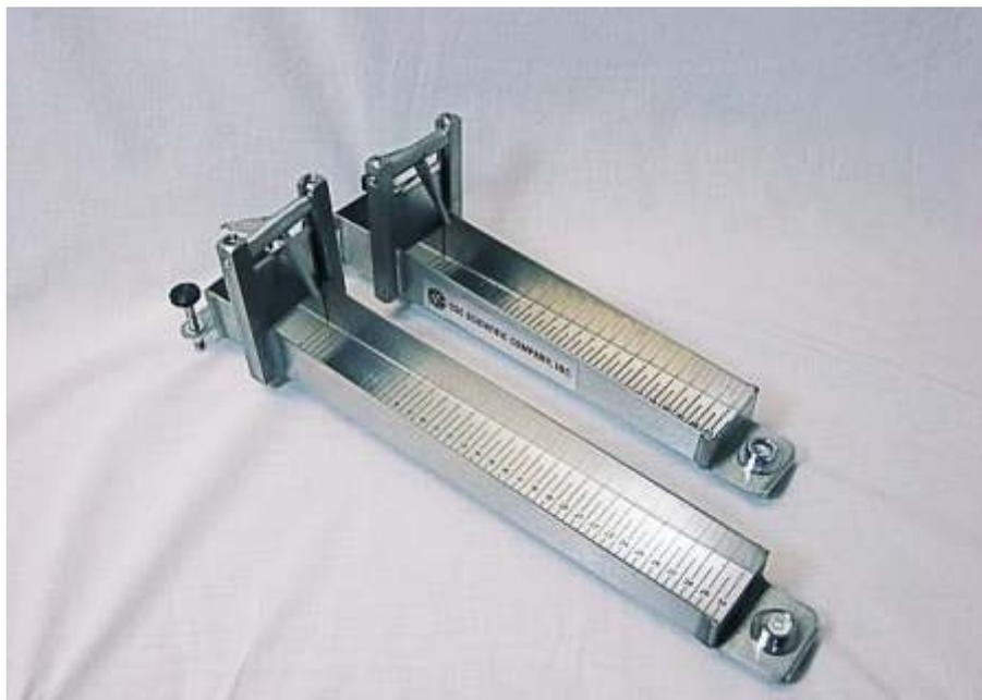
Fig 6.4 Bostwick Consistometer
