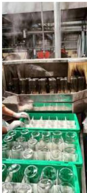
Fig. 7.2 Cleaning and Sterilizing Machine
