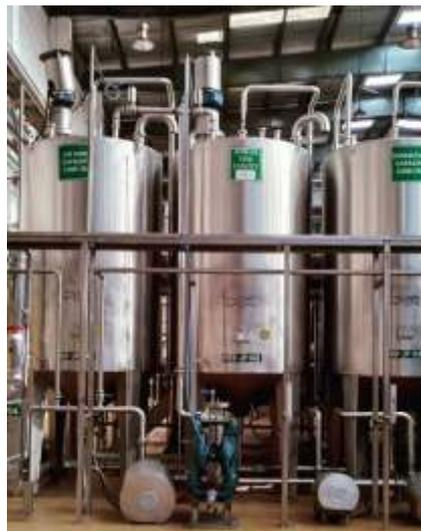
Fig 6.3 Storage Tank for Ketchup Making
