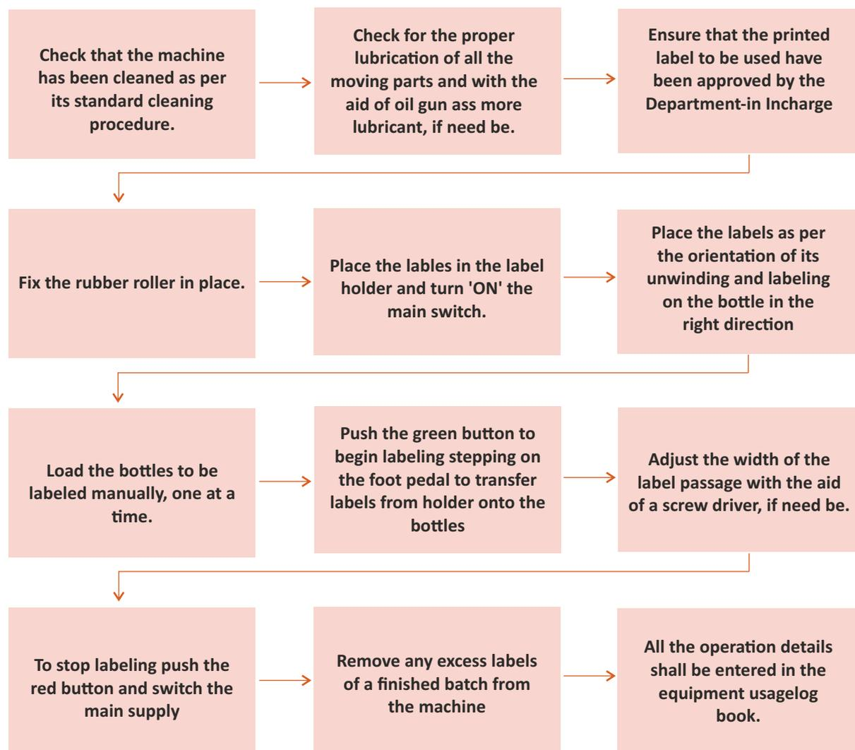
Fig.7.6 Standard Procedure to load labels in labelling machine.
