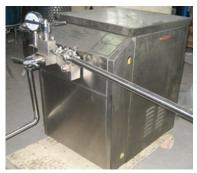
Fig. 1.15: Homogenizer
