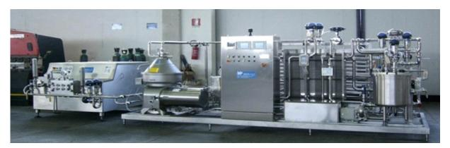
Fig. 1.14: Pasteurization Unit
