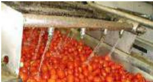
Fig. 6.2.3. High pressure water nozzles
