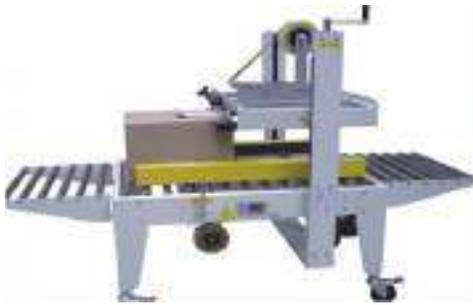
Fig. 6.2.17. Carton packing/strapping machine
