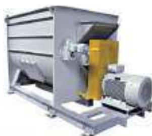
Fig 6.2.11. Mechanical dryers
