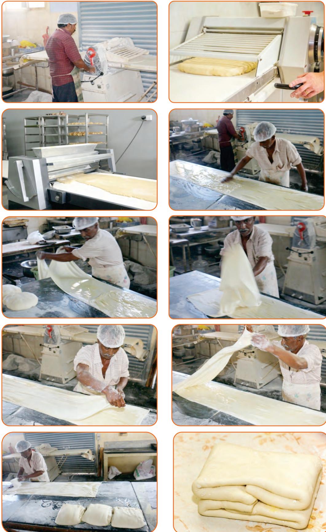
Fig. 5.18 Preparation of laminated pastry dough using laminator
