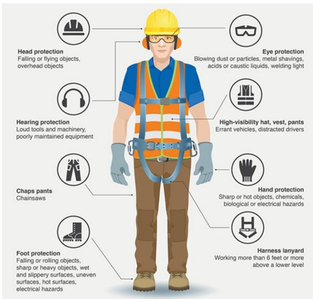
Fig. 5.4.1: The usage of personal protective equipment
